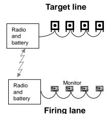
No wire between the target(s) and the firing line
