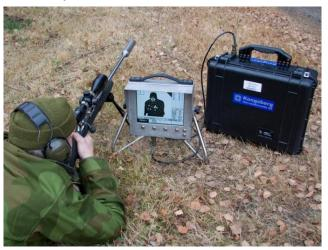
Monitor built on LCD technology with LED backlight, designed for all-year outdoor use. No need for over roofed firing points.
